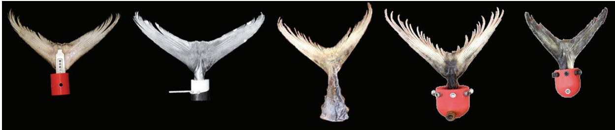
Figure 4.1: The five tail samples used in the biological testing. From left to right, the species are: bigeye, albacore, bigeye, yellowfin, and Spanish mackerel. Fins 1, 2, 4, and 5 are shown mounted into their housings, and the strut used impose the constraint is visible in fin 1.
