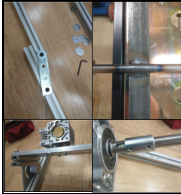
Figure 17: Images showing some key parts of the final rig: the extrudable part of the base (top left), the welding of the shaft (top right), the adjustable mount (bottom left) and the shaft coupling (bottom right).
