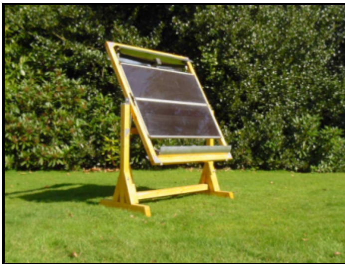
Figure 1: Passive tracker design utilizing two bimetallic strips by Clifford et. al.
