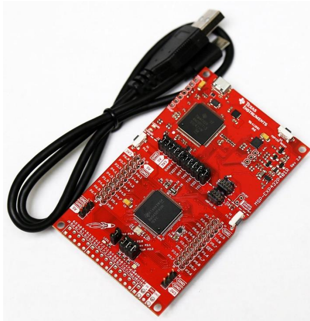
Figure 4. Texas Instruments MSP432P401R Microcontroller
