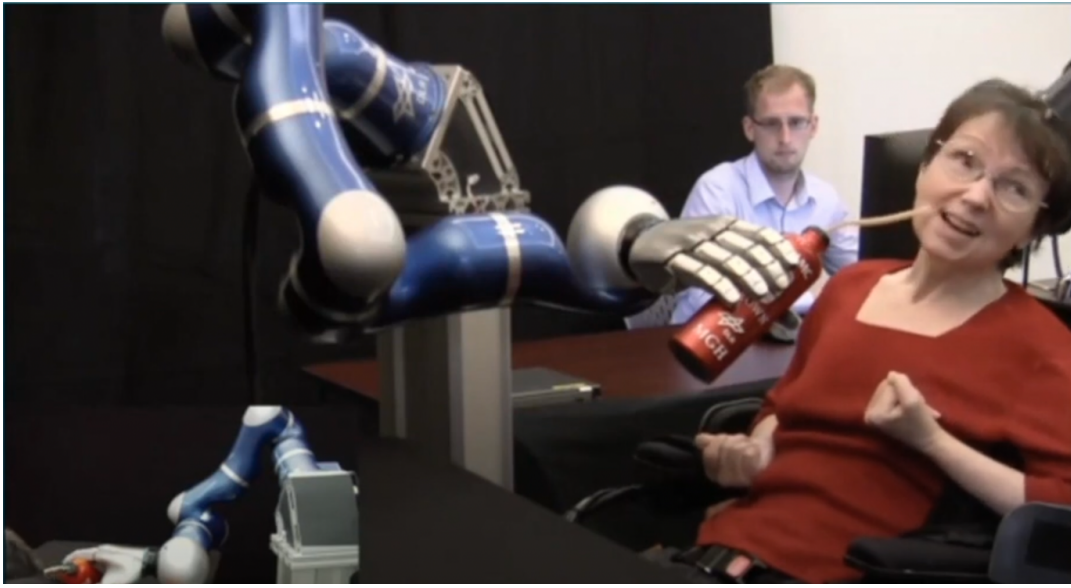
“Drinking from a cup with a neurally controlled assistive robotic device by a person with tetraplegia” (Hochberg & Unite Genomics, Inc., 2021).
