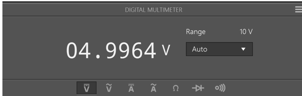
Figure 11: 5V Voltage Regulator Output
