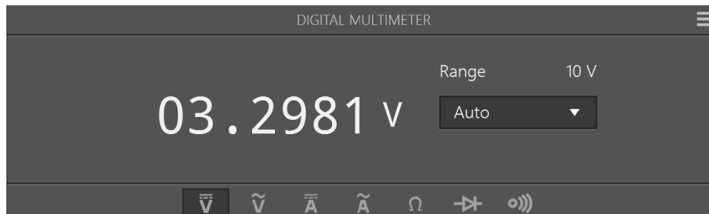
Figure 10: 3.3V Voltage Regulator Output
