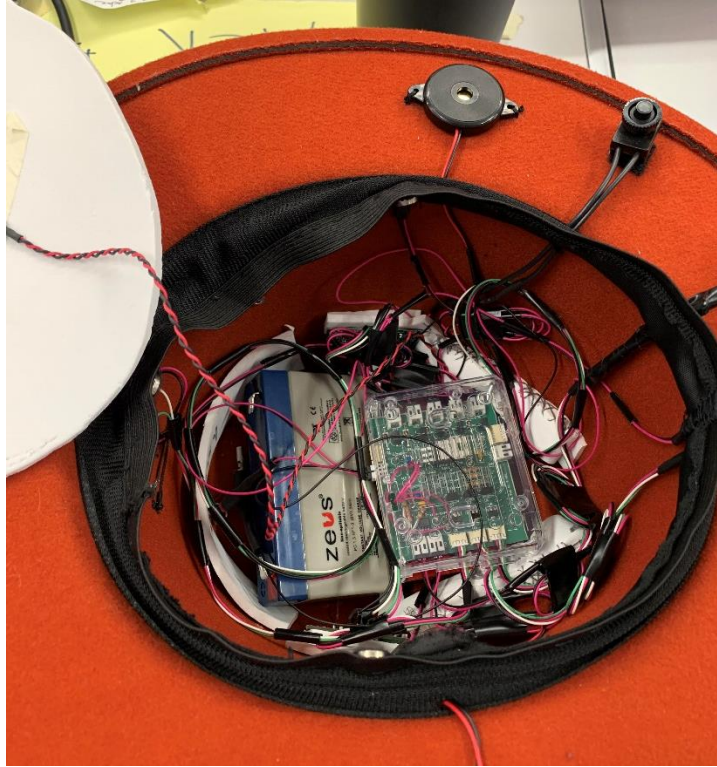
Figure 19: Inside Hat with PCB Casing
