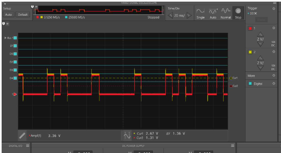
Figure 18: PWM Interrupts Varied Duty Cycle Test
