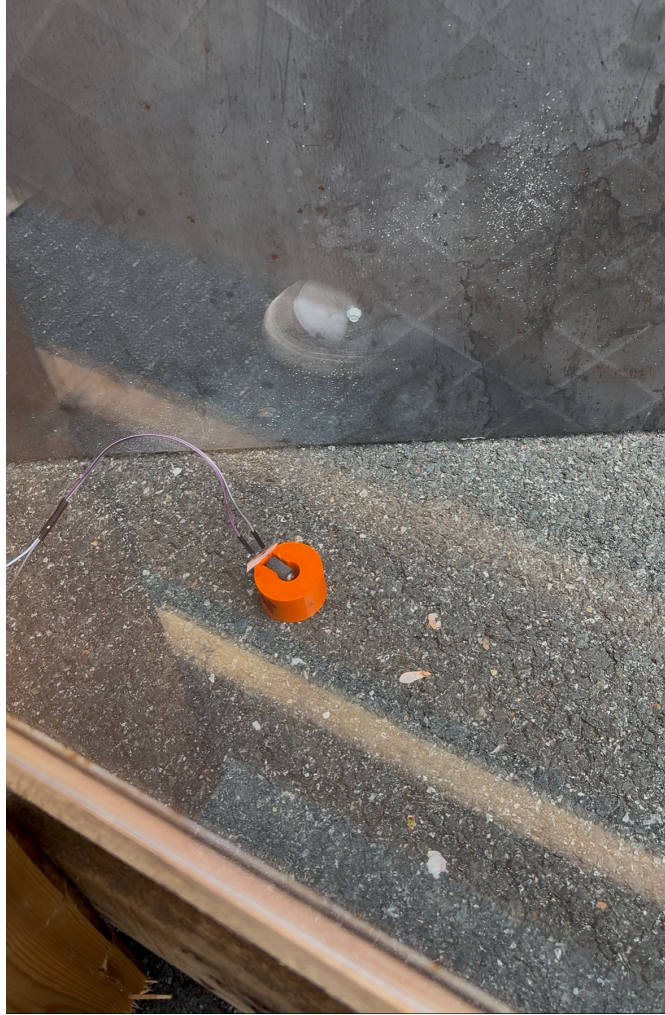
Figure 20: Circular fuel grain With Pyrodex cutout during ignition system testing. Note presence of blast shield with polycarbonate viewing panel.
