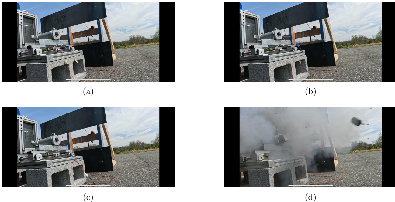
Figure 32: Ignition cables traveling down the engine, indicating failure due to nozzle clogging.
