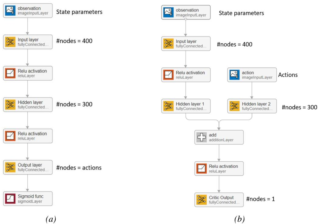
Figure A-1: (a) Actor and (b) Critic network for the DDPG agent coupled with arm MB model for elbow kinematics. The number of nodes at each layer is provided corresponding to the layer.
