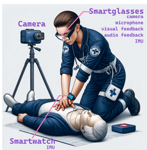
Figure 1.1: Sensors used for a cognitive assistant
