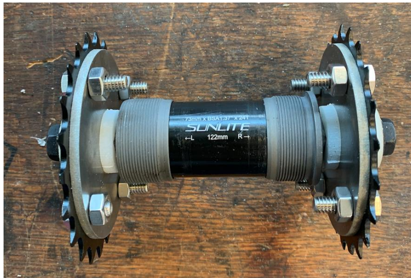
Figure 11: Interstitial Gear before being threaded into its framing.
