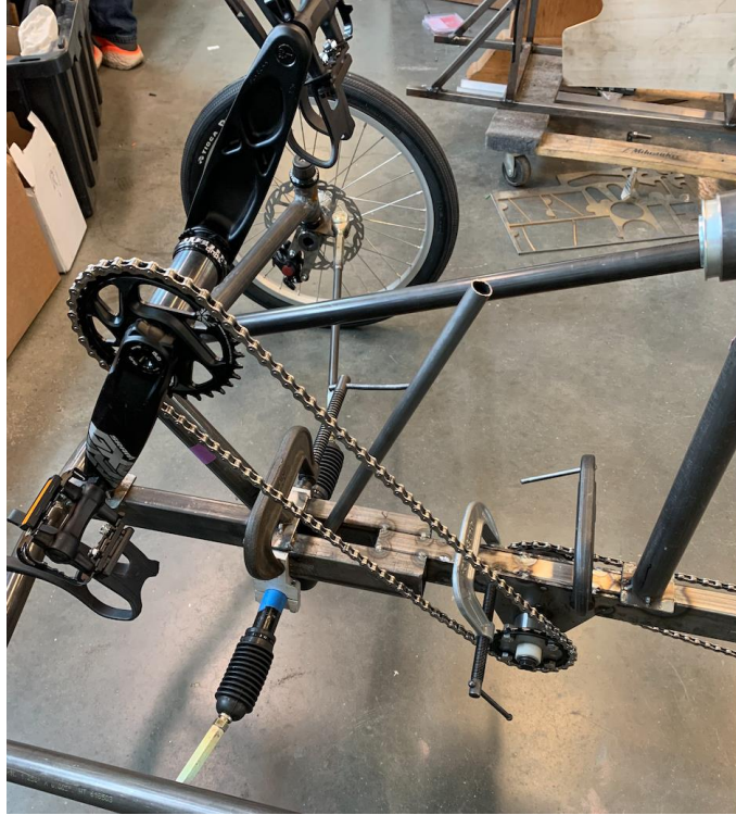
Figure 12: Front half of two-chain system and the 32T chainring.
