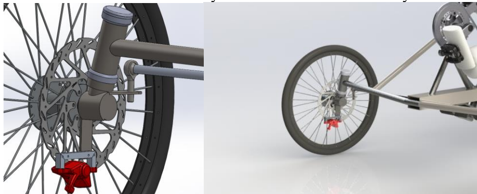
Figure 5. The front-wheel brake assembly mounted on the steering head.
