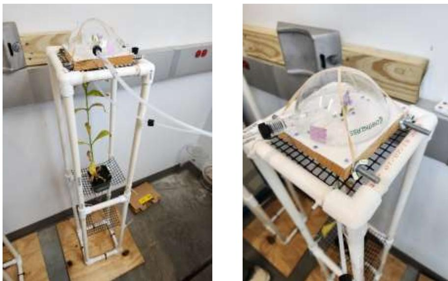
*Figure 5ab. Floral Headspace Guillotine Device. The image on the left (5a) shows the full design of the guillotine with a plant inside to demonstrate the collection. The image on the right (5b) shows the headspace where the florals are filtered out.*
