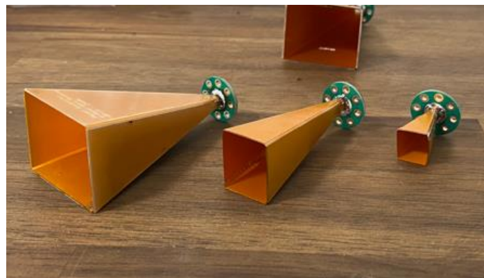
Figure 6. PCB antennas folded and soldered. From left to right, the PCB antennas are 20 dB, 25 dB, and 15 dB. Dimensions were copied from Pasternack datasheets, and represent an accurate replication of the commercial geometry.
