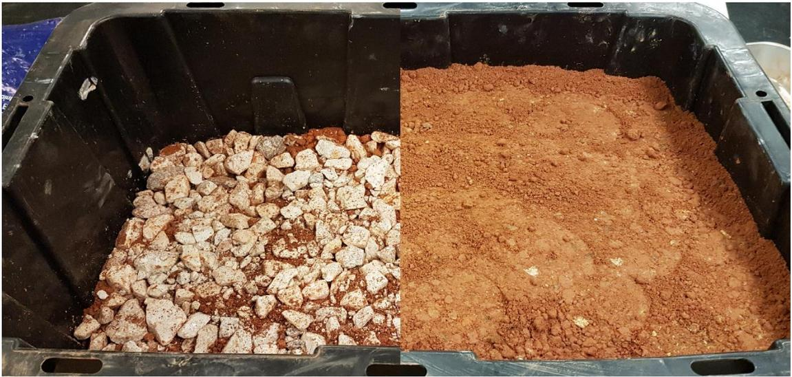
Figure 10. Karst terrain underlain by weathered limestone bedrock reproduced in a tabletop laboratory setting
