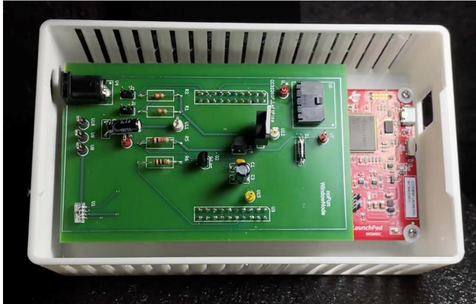
Figure 12: Manufactured Window Node
