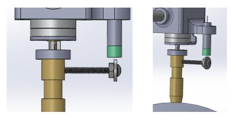
Figure 17. Earth spin motor homing apparatus. The proximity sensor can move up and down using the hex nuts that accompany it. The washer
