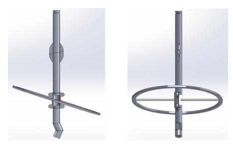
Figure 3. CAD of our first prototype, which used a ring to handle the lunar position
