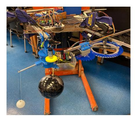
Figure 14. Final physical assembly. Moon-Earth system on the left and Earth orbit system on the right. Note that the 24" lazy susan bearing and hollow 0.5" shaft diameter slip ring were both never delivered. Therefore, we couldn't cantilever the Earth-Moon system as seen in the SolidWorks assembly.
