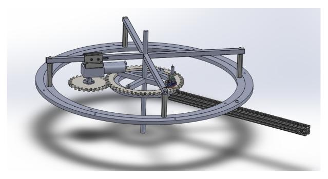
Figure 9. Final Earth orbit assembly in SolidWorks.
