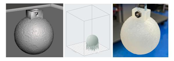
Figure 23. Moon model in Meshmixer (left), Moon model and support structure in Preform (center), 3D printed resin Moon (right)
