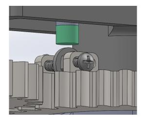
Figure 16. Lunar arm gear with hardware mount (left) and lunar arm motor homing apparatus (right). The slots on the gear allow the washer to move towards/away from the sensor hold. The washer can move along the screw it is on by moving the nuts that secure it. The proximity sensor can move up and down using the hex nuts that accompany it.
