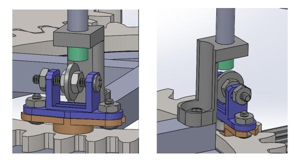
Figure 15. Central driving motor homing apparatus. The blue and orange parts as well as the gray zigzag shaped piece are 3D printed. The green-tipped piece is the inductive proximity sensor. The blue piece has slots to move the washer towards/away from the sensor hold. The washer can move along the screw it is on by moving the nuts that secure it. The proximity sensor can move up and down using the hex nuts that accompany it.
