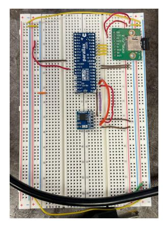
Figure 22. Circuit used to transfer data from SD card to Serial Flash Memory chip
