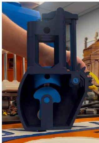
Figure 1: Final 3-D printed four-stroke engine model
