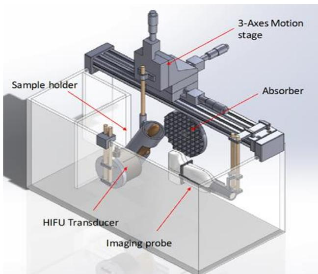
**Figure 7. Schematic of FUS system used:** The FUS system employed here used a tank of degassed water maintained at 37°C. A 1 MHz high intensity focused ultrasound (HIFU) transducer was positioned to treat PCR tubes positioned in the sample holder. The 3-axes motion stage permitted movement of the sample holder so that tubes could be precisely positioned and held steady in the focal point of the transducer. The imaging probe and absorber were not used in these experiments.
