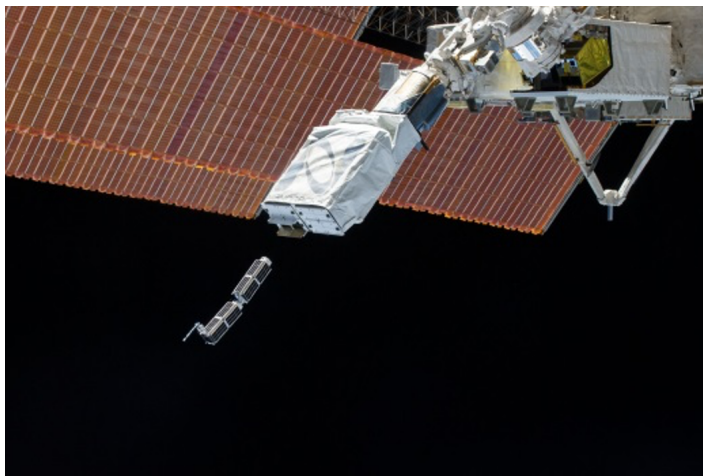
Figure 3. CubeSat launcher on the ISS (Goyne, 2022)
