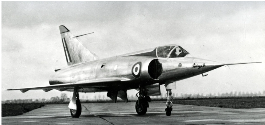
Figure 1.1: Mirage III right-side profile displaying Pitot tube [1]
