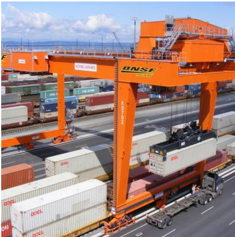
Figure 1. Rail Mounted Gantry Crane made by Konecranes. (Konecranes, 2019)
