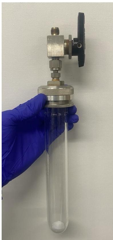
**Figure 2.10.** Photograph of a custom-built high pressure reaction vessel used for photolytic reactions.
