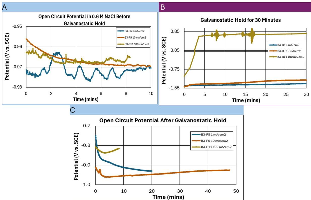
**Fig. 4. A) OCP of sample B3-R5, blue line, sample B3-R16, orange line, and sample B3-R11, dark yellow line. B) Galvanostatic hold of 1 mA/cm<sup>2</sup> on sample B3-R5, blue line. Galvanostatic hold of 10 mA/cm<sup>2</sup> on sample B3-R16, orange line. Galvanostatic hold of 100 mA/cm<sup>2</sup> on sample B3-R11, dark yellow line. C) OCP after galvanostatic hold, of sample B3-R5, blue line, sample B3-R16, orange line, and sample B3-R11, dark yellow line.**
