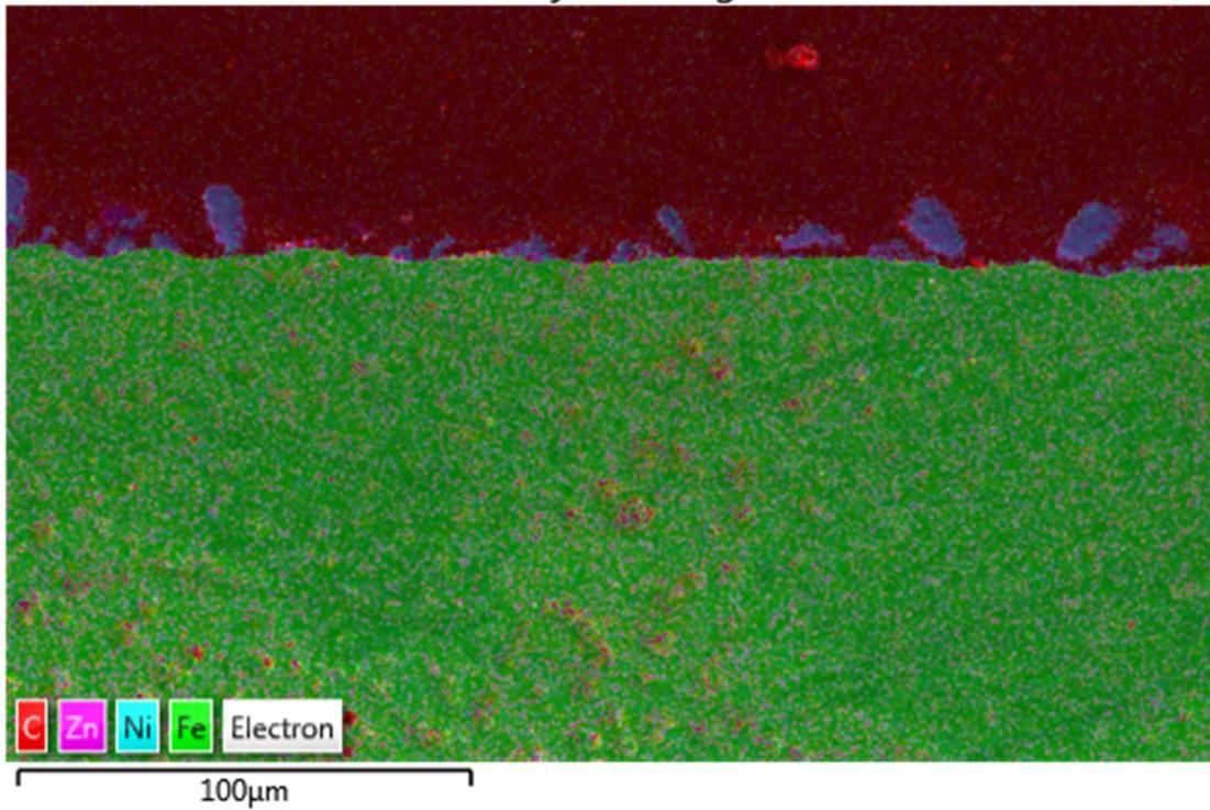
Fig. 29. Sample B3-R28 was taken to EDS after selective dissolution and there was not a continuous Zn-Ni coating left on the surface. This is shown in this compositional map.
