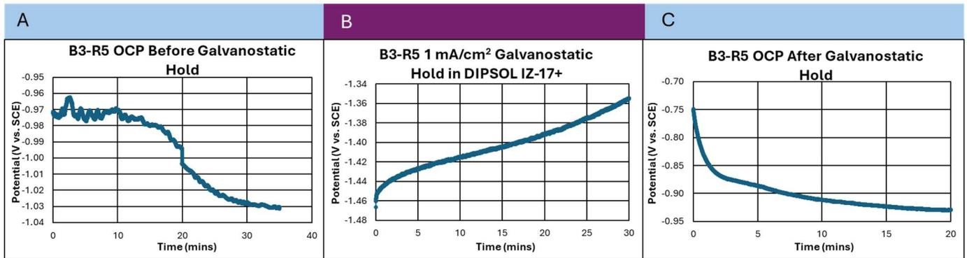
**Fig. 17. Sample B3-R5 A) OCP in 0.6 M NaCl before galvanostatic hold; B) The change in potential due to the galvanostatic hold of 1 mA/cm<sup>2</sup> for thirty minutes in DIPSOL IZ-C17+; C) OCP in 0.6 M NaCl after galvanostatic hold.**
