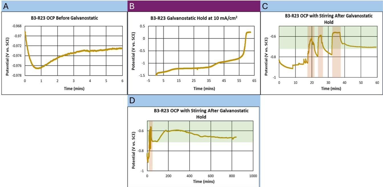
**Fig. 6. Sample B3-R23 A) OCP in 0.6 M NaCl before galvanostatic hold; B) The change in potential due to the galvanostatic hold of 10 mA/cm<sup>2</sup> for 62 minutes in DIPSOL IZ-C17+; C) The first 60 minutes of the OCP technique in 0.6 M NaCl, including the sections of stirring at 900 RPM; D) The extended view of the 13 hour long OCP technique to test the impact of stirring in the 0.6 M NaCl after the galvanostatic technique.**
