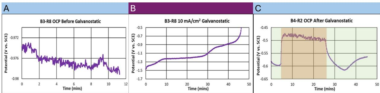
**Fig. 8. Sample B3-R8 A) OCP in 0.6 M NaCl before galvanostatic hold; B) Change in potential due to the galvanostatic hold of 10 mA/cm<sup>2</sup> until the 0.5 V vs. SCE potential limit in DIPSOL IZ-C17+; C) OCP in 0.6 M NaCl, with 20 minutes of stirring, after the galvanostatic hold.**
