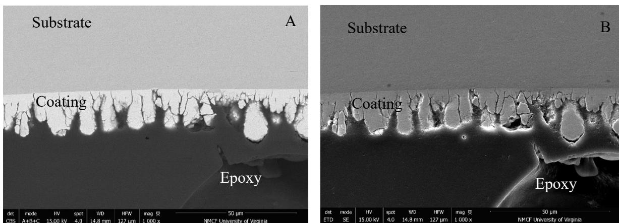
**Fig. 11. Sample B3-R5 displays the columnar structure that is a characteristic of a coating applied by electrochemical deposition, seen in A) BSE micrograph and B) SE micrograph.**
