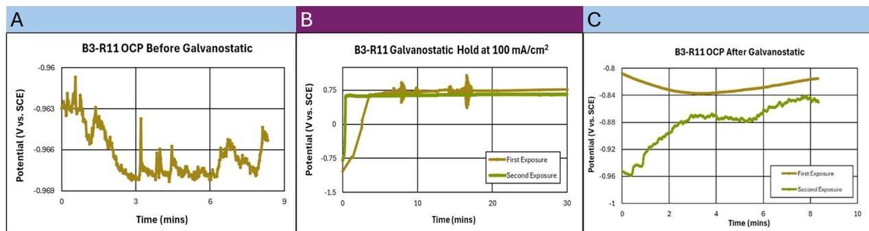
**Fig. 5. Sample B3-R11 A) OCP in 0.6 M NaCl before galvanostatic hold; B) The change in potential due to the galvanostatic hold of 1 mA/cm<sup>2</sup> for thirty minutes in DIPSOL IZ-C17+, with repeated exposures; C) OCP in 0.6 M NaCl after the first and second galvanostatic hold.**
