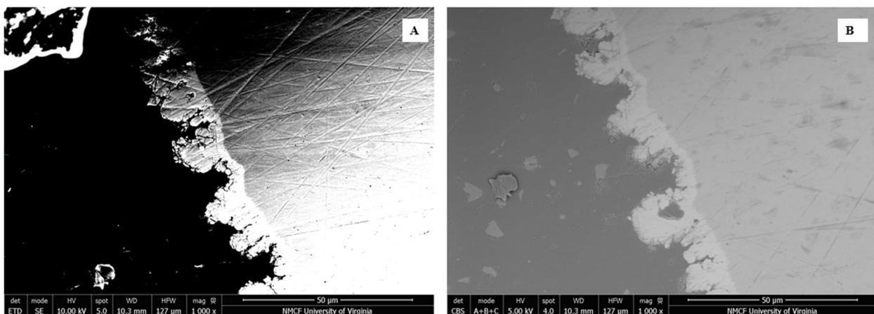
**Fig. 13. Sample B3-R2 SEM micrographs: a) Zn-Ni coating cross section ETD at 1000x b) Zn-Ni coating cross section CBS at 1000x.**
