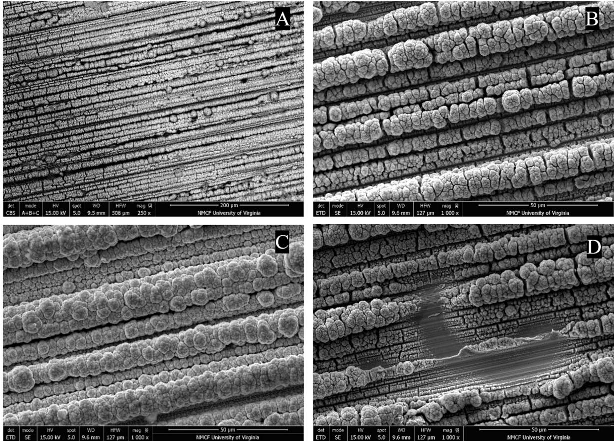
**Fig. 22. A) BSE micrograph of B3-R11's the transition region from unexposed region to exposed region at 250x. B) SE micrograph of B3-R11's unexposed region at 1000x. C) SE micrograph of B3-R11's exposed region at 1000x. Secondary electron (SE) micrograph of point of interest on B3-R11 at 1000x. All micrographs are in plan view and done after the sample's second exposure.**
