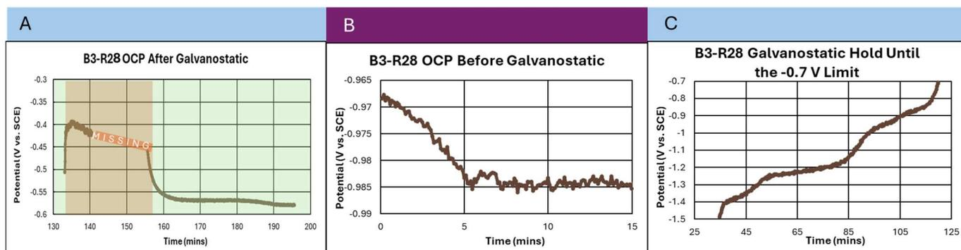
**Fig. 26. Sample B3-R28 A) OCP in 0.6 M NaCl before galvanostatic hold; B) Change in potential due to the galvanostatic hold of 10 mA/cm<sup>2</sup> until the 0.7 V vs. SCE potential limit in DIPSOL IZ-C17+; C) OCP in 0.6 M NaCl, with 20 minutes of stirring, after the galvanostatic hold.**
