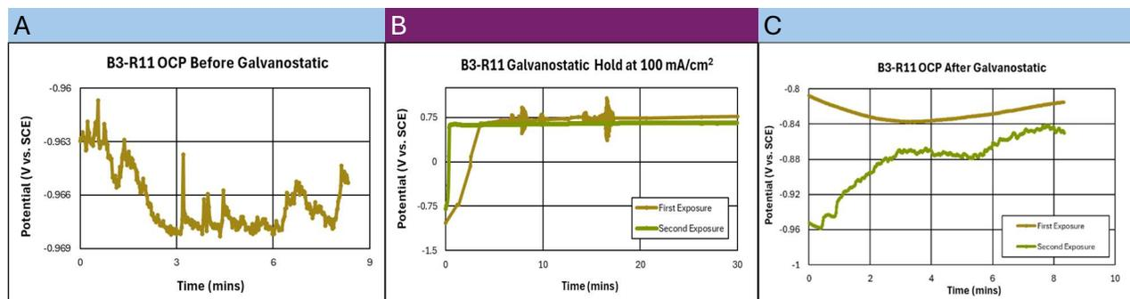
**Fig. 5. Sample B3-R11 A) OCP in 0.6 M NaCl before galvanostatic hold; B) The change in potential due to the galvanostatic hold of 1 mA/cm<sup>2</sup> for thirty minutes in DIPSOL IZ-C17+, with repeated exposures; C) OCP in 0.6 M NaCl after the first and second galvanostatic hold.**
