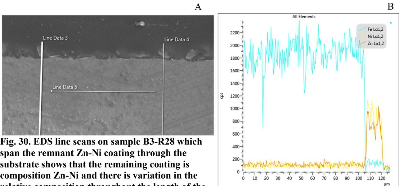
Fig. 30. EDS line scans on sample B3-R28 which span the remnant Zn-Ni coating through the substrate shows that the remaining coating is composition Zn-Ni and there is variation in the relative composition throughout the length of the remnant Zn-Ni.
