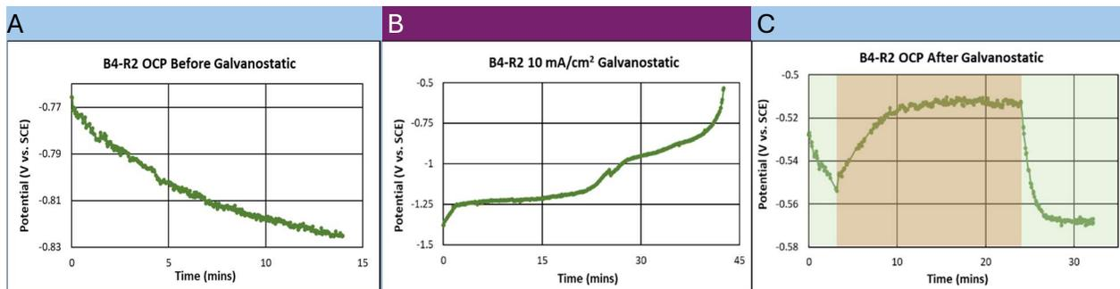
**Fig. 9. Sample B4-R2 A) OCP in 0.6 M NaCl before galvanostatic hold; B) Change in potential due to the galvanostatic hold of 10 mA/cm<sup>2</sup> until the 0.5 V vs. SCE potential limit in DIPSOL IZ-C17+; C) OCP in 0.6 M NaCl, with 20 minutes of stirring, after the galvanostatic hold.**
