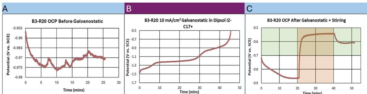
**Fig. 7. Sample B3-R20 A) OCP in 0.6 M NaCl before galvanostatic hold; B) Change in potential due to the galvanostatic hold of 10 mA/cm<sup>2</sup> until the 0.5 V vs. SCE potential limit in DIPSOL IZ-C17+; C) OCP in 0.6 M NaCl, with 20 minutes of stirring, after the galvanostatic hold.**
