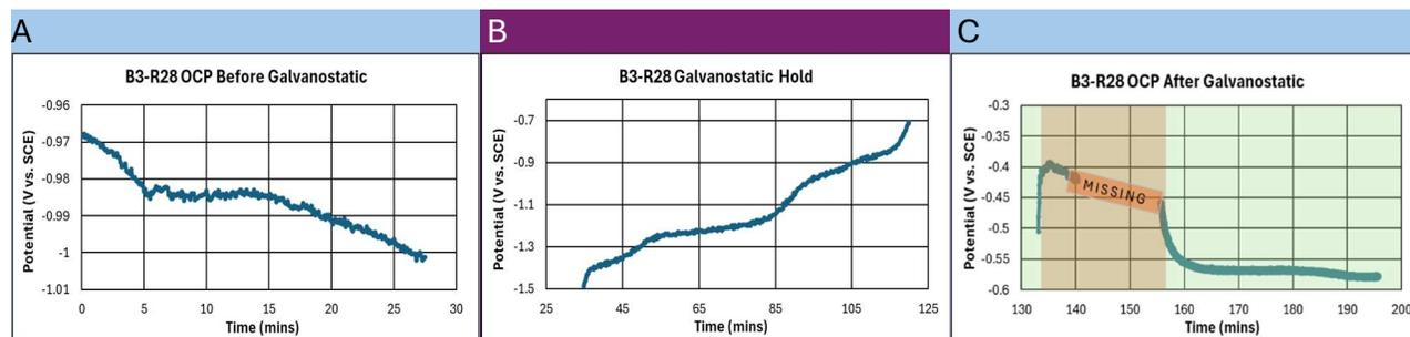
**Fig. 10. Sample B3-R28 A) OCP in 0.6 M NaCl before galvanostatic hold; B) Change in potential due to the galvanostatic hold of 10 mA/cm<sup>2</sup> until the 0.7 V vs. SCE potential limit**
