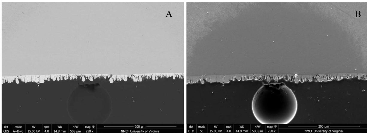
**Fig. 18. Sample B3-R5 cross-sectional SEM micrographs display that the coating structure is consistent on the surface of the substrate after electrochemical selective dissolution technique A) BSE B) SE.**
