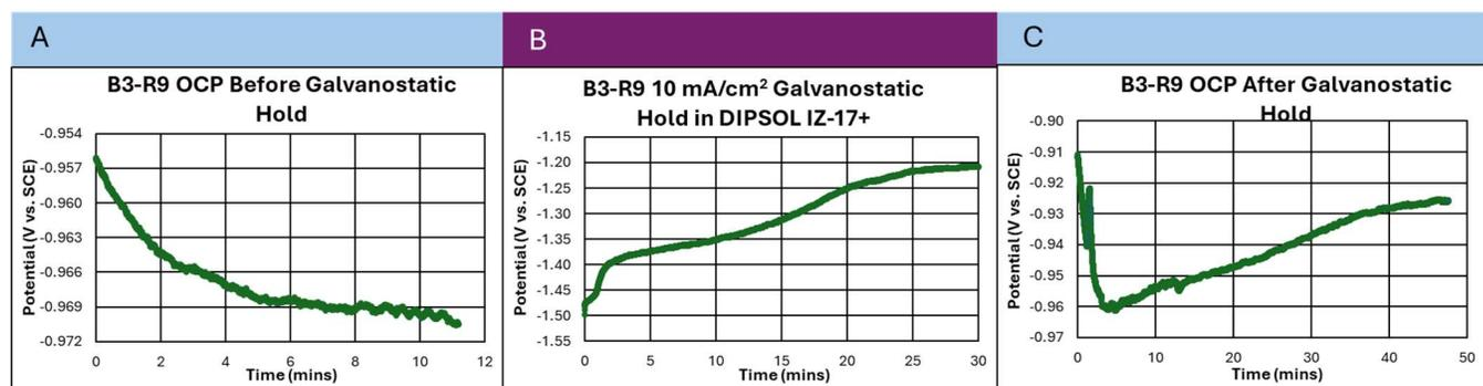
**Fig. 20.** Sample B3-R9 A) OCP in 0.6 M NaCl before galvanostatic hold; B) Change in potential due to the galvanostatic hold of 10 mA/cm<sup>2</sup> for 30 minutes in DIPSOL IZ-C17+; C) OCP in 0.6 M NaCl after galvanostatic hold.
