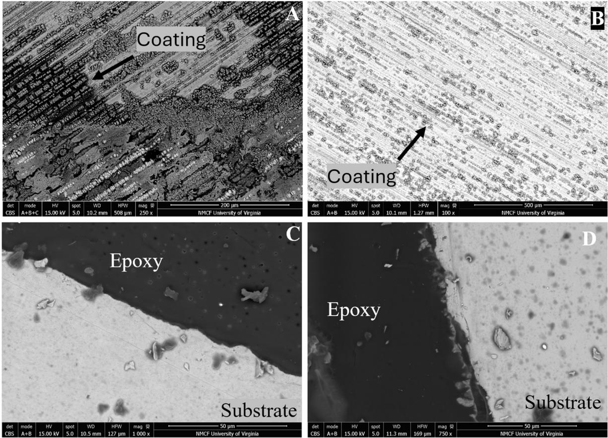
**Fig. 24. A) BSE micrograph (CBS with ABC) of B3-R20 at 250x along edge of corrosion circle. B) B3-R23 plan view at 100x in the center of the corrosion circle. C) B3-R20 cross-section at 1000x. D) BSE micrograph of B3-R23 cross-section at 750x.**
