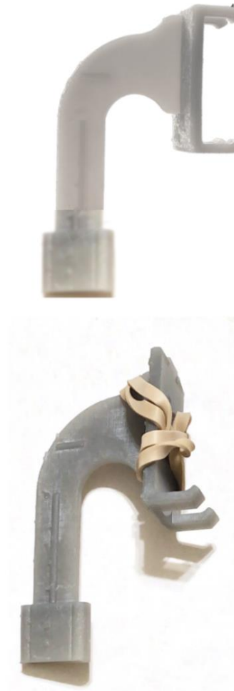
Figure 2. Novel positioning device: This is the device that we designed, 3D printed, and used for our testing trials.
