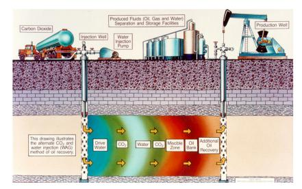
Diagram of water alternating gas injection (Al-Netaifi, 2008).
