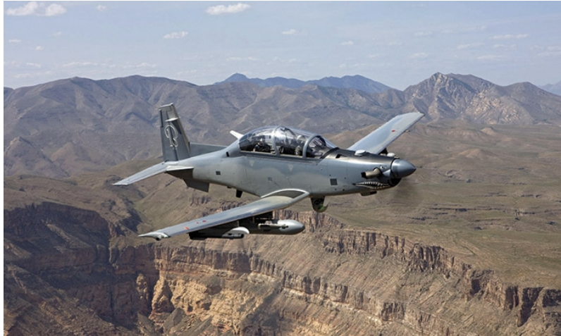
Figure 1: AT-6 Wolverine in flight, notice the low wing design and the numerous missile and bombs connected to the hardpoint for ground strikes ( AT-6 Wolverine , n.d.)
