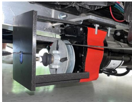
Figure 1: DC motor used on Cart 788 to pull the braking cable.
