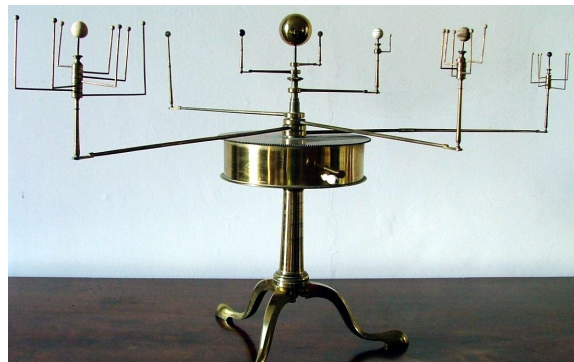
Figure 1. Traditional mechanical orrery (Williams, 2016)
