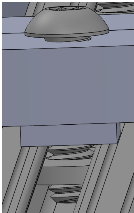
Figure 10. Close-up of the connection between the outer track of the lazy susan and the 80-20 aluminum arm.
