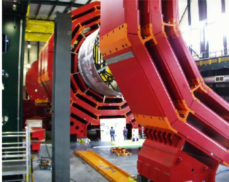
Figure 3.8: A photo of a yoke endcap disk, the central wheel with the vacuum tank, and an additional barrel wheel during magnet assembly in SX5.[44]
