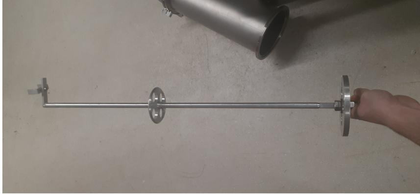
Figure 7: The metal apparatus used to hold target material in the beamline.
