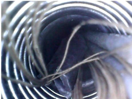
(b) Waveguide Half extracted from Bellows
