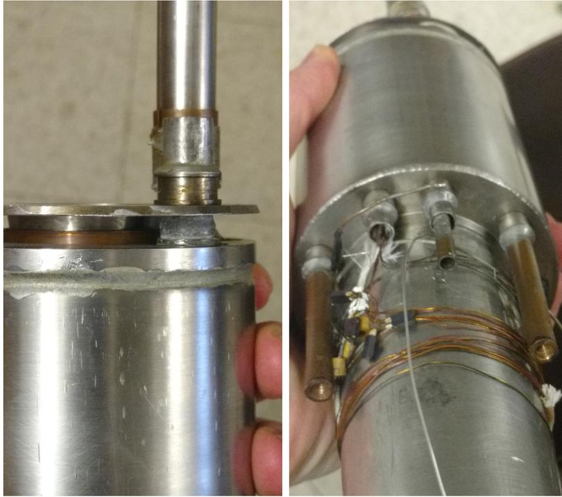
(a) Upstream Face of Still Exposed (b) Inside of Still with Heater and Pumpout shown
