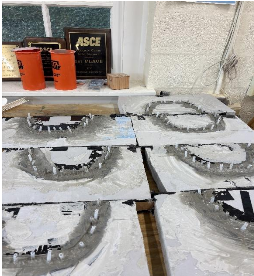
Figure 6: Concrete Placed in Molds
