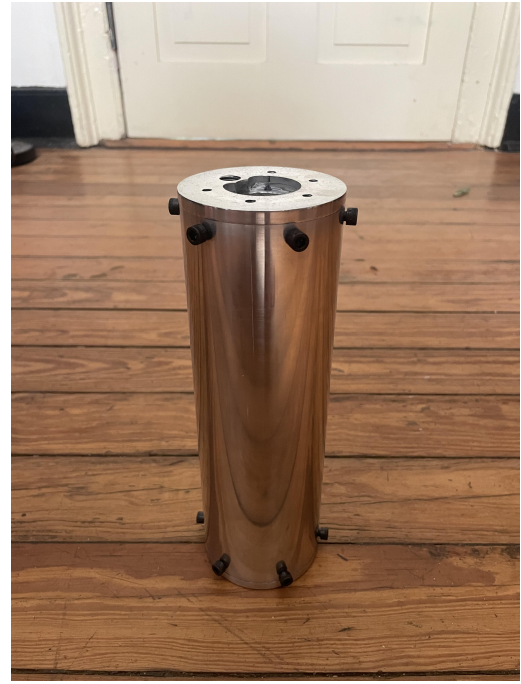
(b) ATLAS II combustion chamber before testing.
