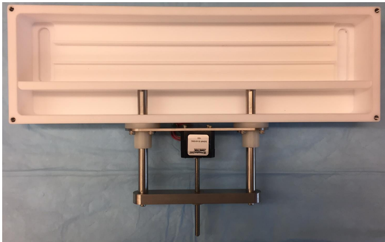
Figure 2.1.3 , Bioreactor Body, Translating Arm, and Motor
