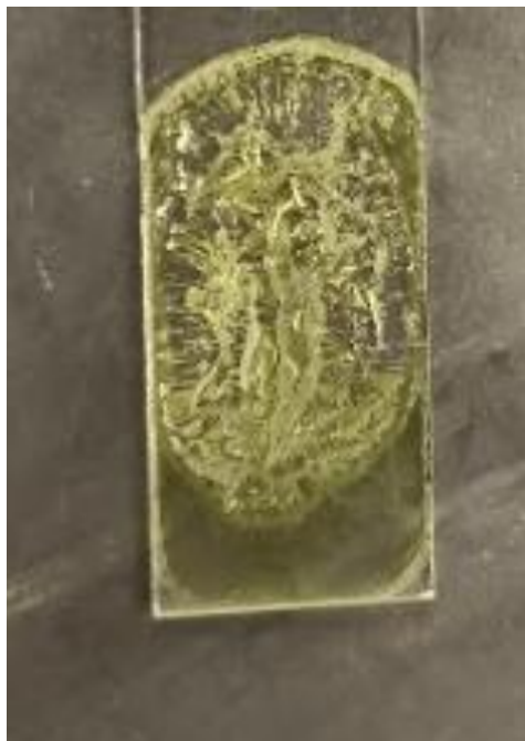
Figure A3.1. Optical image of the NU-901 film drop casted at 140 °C. (For this condition, solvent is DMSO, \text{ZrOCl}_2 \cdot 8\text{H}_2\text{O} concentration is 35.4 mM, \text{H}_4\text{TBAPy} concentration is 6.8 mM, and formic acid concentration is 1.9 M)
