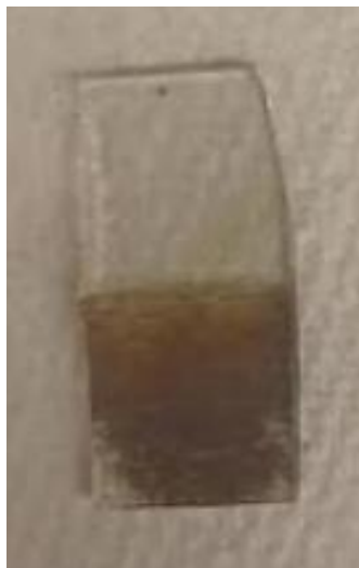
Figure A3.15. Optical image of the MOF-525 film synthesized at 180 °C using solution shearing. (For this condition, solvent is DMSO, \text{ZrOCl}_2 \cdot 8\text{H}_2\text{O} concentration is 35.4 mM, TCP concentration is 14.1 mM, formic acid concentration is 1.9 M, and blade speed is 0.025 mm/s)
