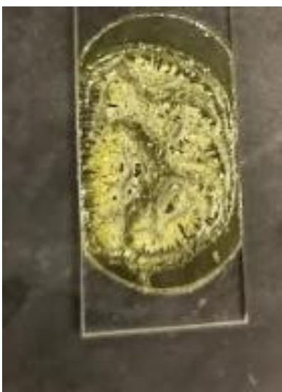
Figure A3.2. Optical image of the NU-901 film drop casted at 160 °C. (For this condition, solvent is DMSO, \text{ZrOCl}_2 \cdot 8\text{H}_2\text{O} concentration is 35.4 mM, \text{H}_4\text{TBAPy} concentration is 6.8 mM, and formic acid concentration is 1.9 M)
