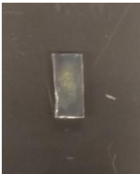
Figure A2.6. Photo of NU-1000 thin film after being sonicated for three minutes. Reprinted with permission from ref. [60]. Copyright 2020 American Chemical Society.
