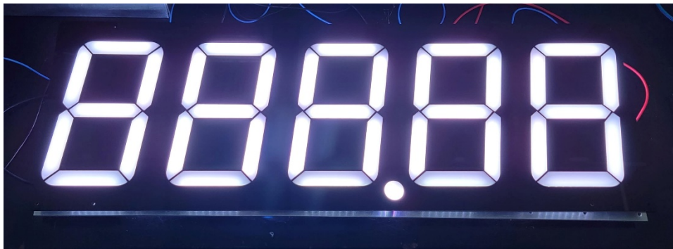
Fig. 2.10.7. Complete LED Backlit Acrylic
