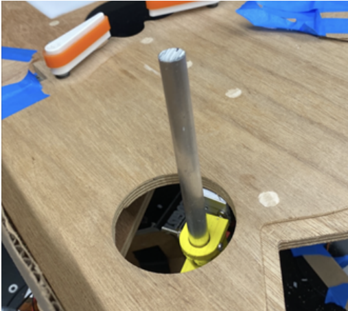
Fig. 2.3.4. First iteration of pop bumper mounted to playfield (top view)
