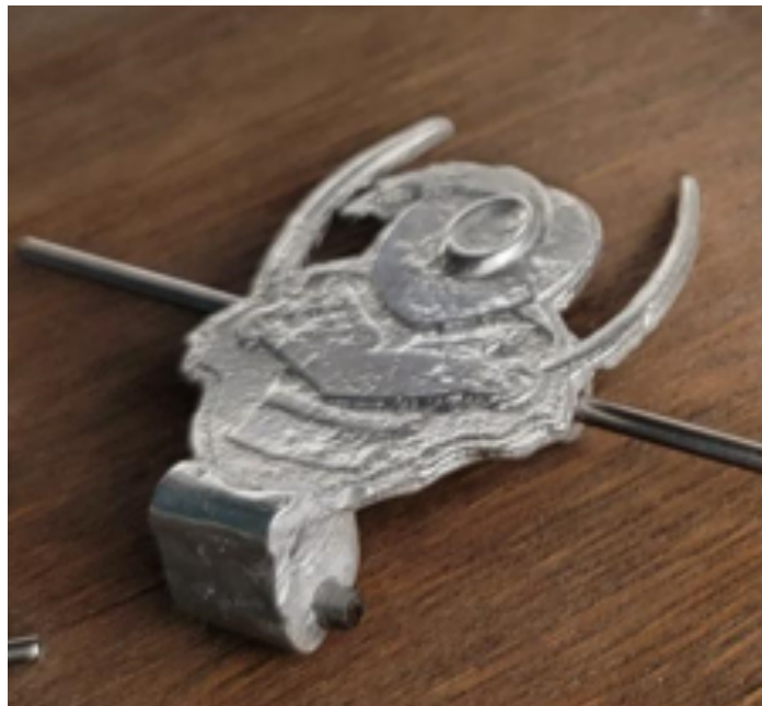
Fig. 2.8.5. Final sand-casted version of the Cavman spinner with tungsten weight
