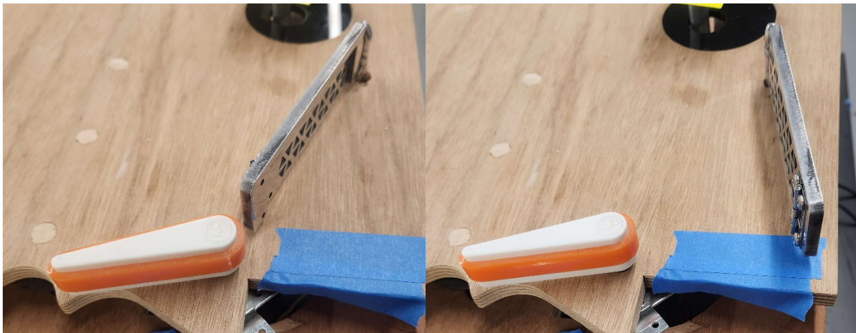
Fig. 2.5.2. Diverter gate in closed and open position
