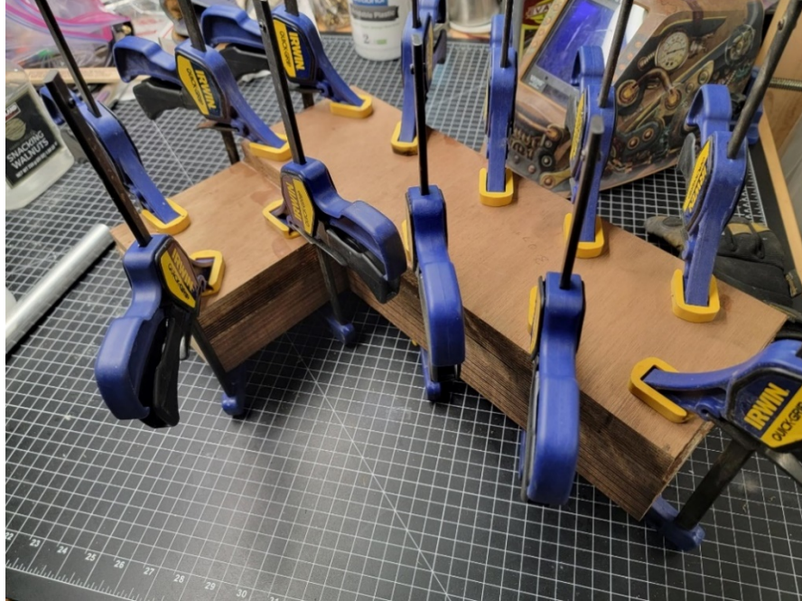
Fig. 3.3.4. Upper Playfield Plywood Stock Glued
