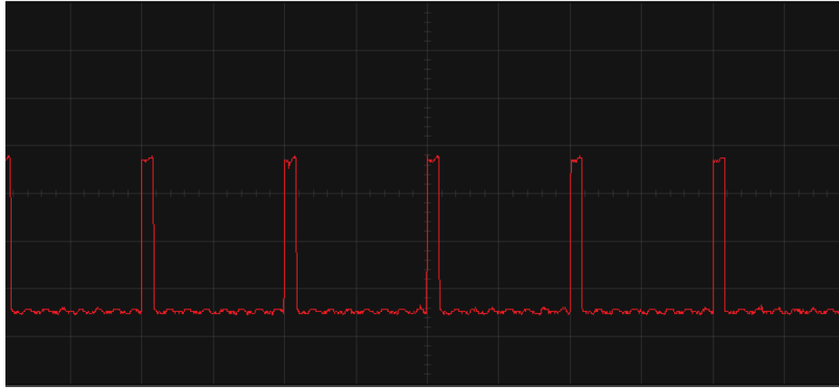
Figure 43 Servo Signal with Motor Running
