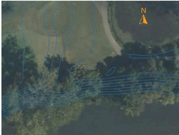
Figure 11: Headcut Survey Data with existing contours
