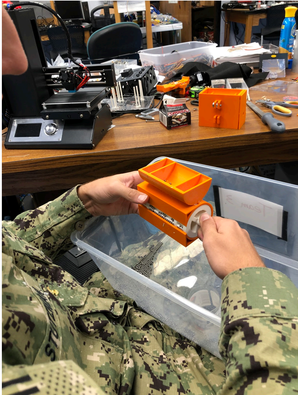
Figure 13: Spinning a preliminary model of the reservoir-drum assembly
