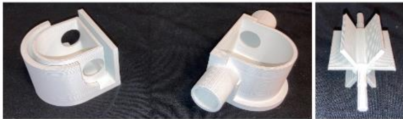
Figure 7: 3D Printed Parts of the Gas Flow Indicator from the Stratasys Printer using ASA Filament
