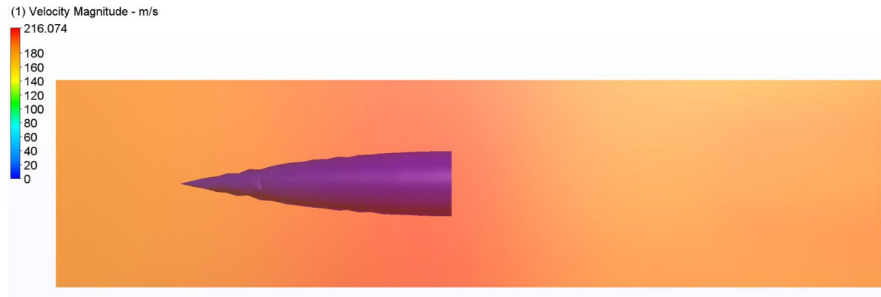
Figure 9. CFD results from Autodesk CFD for chosen nosecone design.
