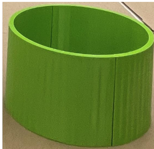
Figure 55. Extended nosecone mold (Height 10 cm)
