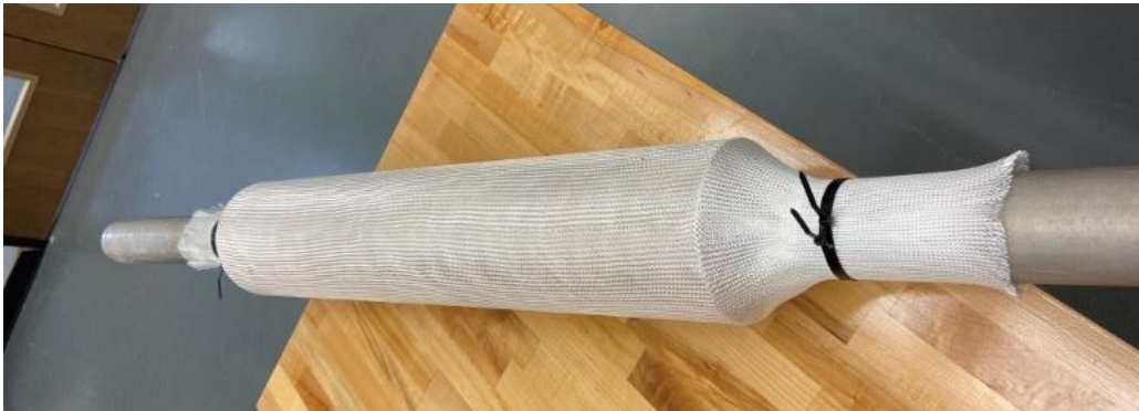
Figure 63. Fiberglass sleeve fixed over phenolic tubing.
