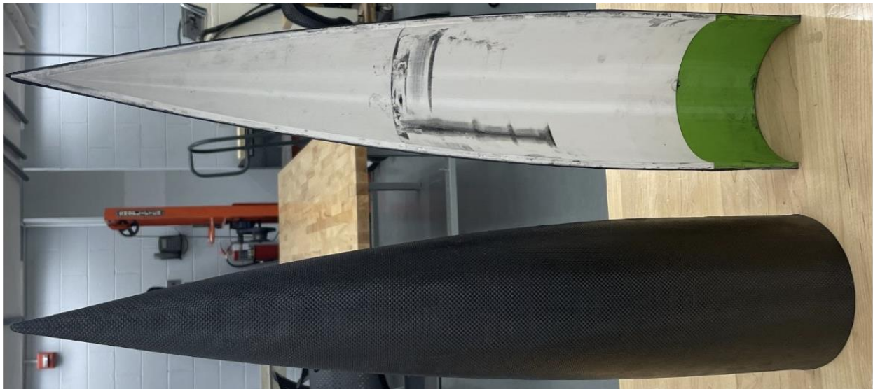
Figure 57. After 3 layers of CFRP wet layup
