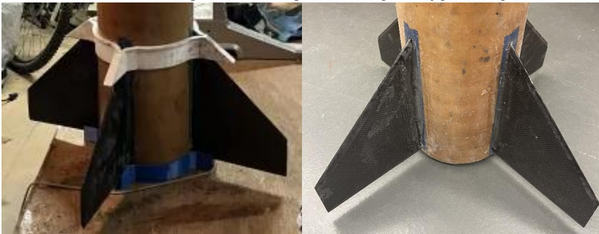
Figure 61. Fins in the slots aligned and hardening with the 3D printed fin alignment jig
