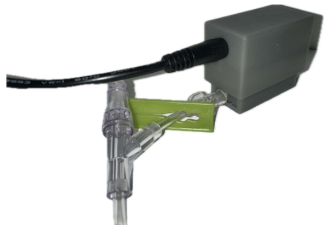
Figure 7. Alternate view of final prototype of housing, cartridge, and power supply with other connection to central line tubing.
