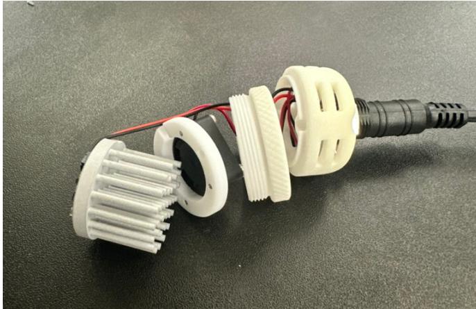
Figure 1. Disassembled mini-UV unit from AquiSense. Components from left to right are UV light attached to heat sink, fan, and connection to power supply.
