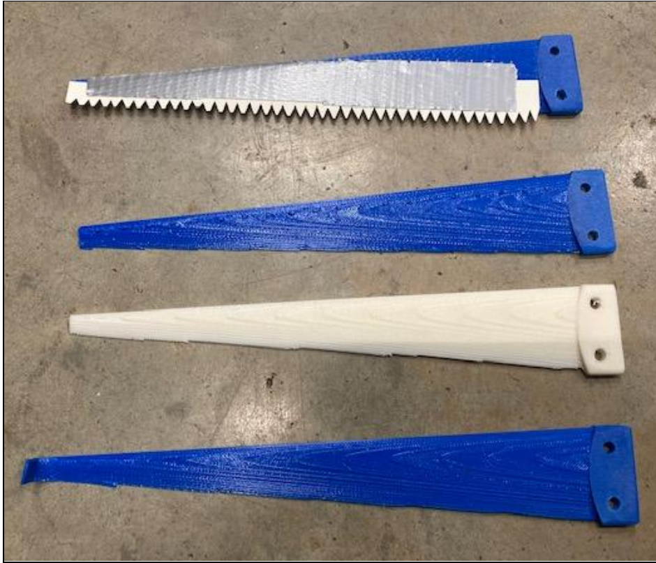
Figure 5. The final set of modified blade prints; pictured from top to bottom: serrations, nodes, base, winglets.
