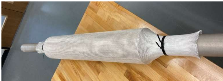
Figure 63. Fiberglass sleeve fixed over phenolic tubing.
