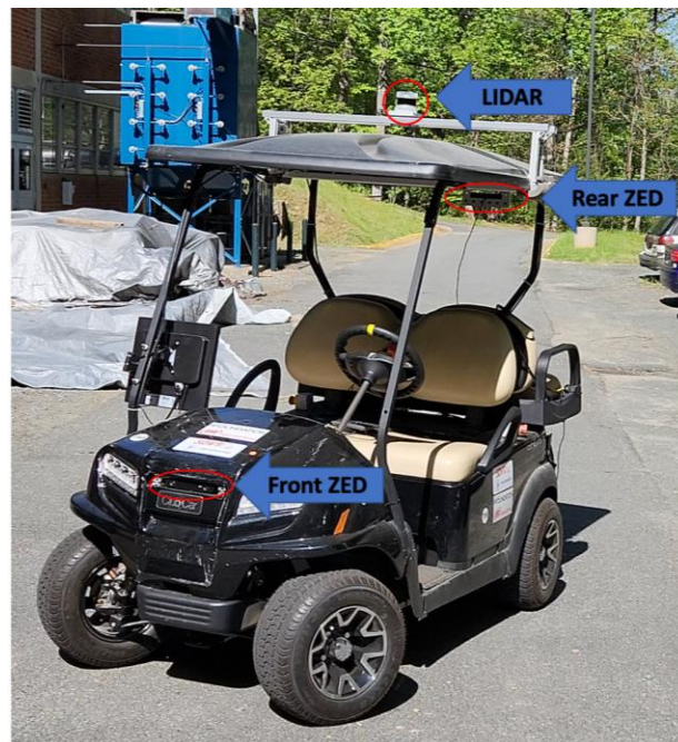
Figure 18: A depiction of the layout of the sensors.
