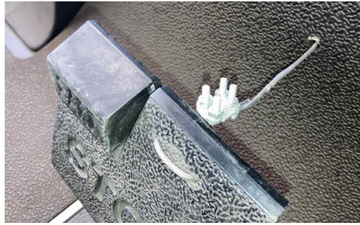
Figure 2: Attachment of the airline cable to the brake pedal of Cart 788 that allows for the pedal to be pulled when the brake motor is engaged.
