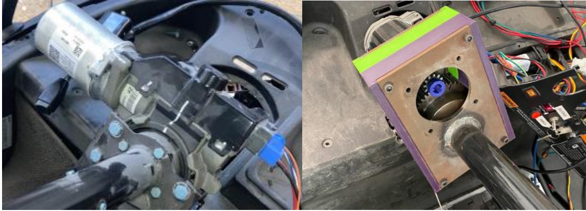
Figure 3 : Nexteer electric power steering system (left); Teknic ClearPath Servo Motor with gears housed in an enclosure (right).
