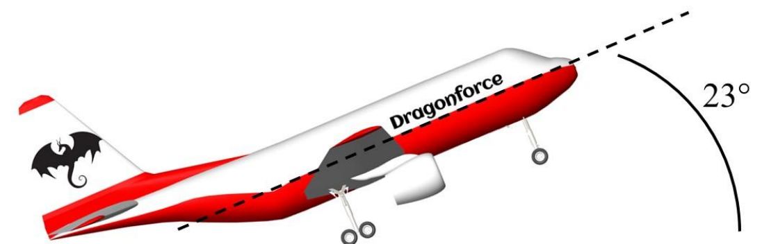
Figure 12-9. Dragonforce Maximum Takeoff Angle
