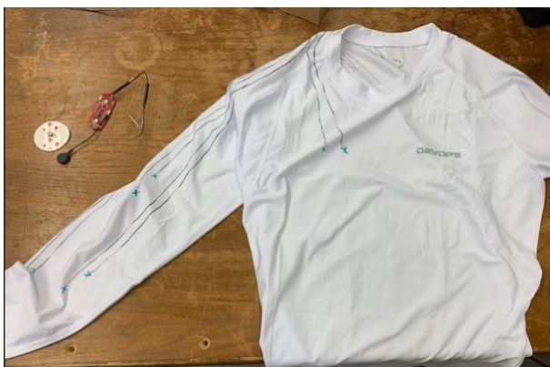
Fig. 8. Planned design for the textile version of the EMG gel electrodes and wiring connections
