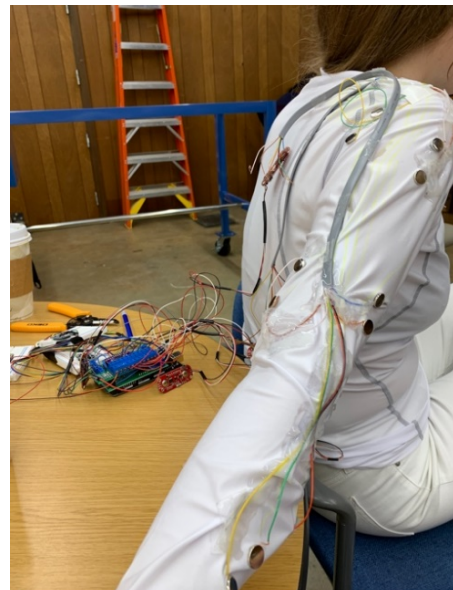
Fig. 9. The textile version of the sensor array depicts the snap connectors to gel electrodes, rainbow wire cables, sensor array, and wire-to-fabric stabilizing glue and tape
