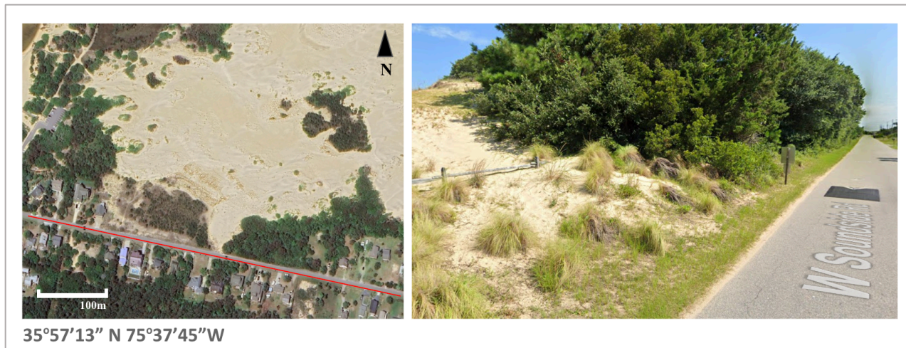
Figure 4. Two perspectives of Soundside Road and the nearby infrastructure. An aerial view (left) shows the road marked in red and the dunefield to the north. A street view (right) shows the sand bypassing a fence and approaching the road. Image source: Google Earth / Airbus, 4/25/2023.
