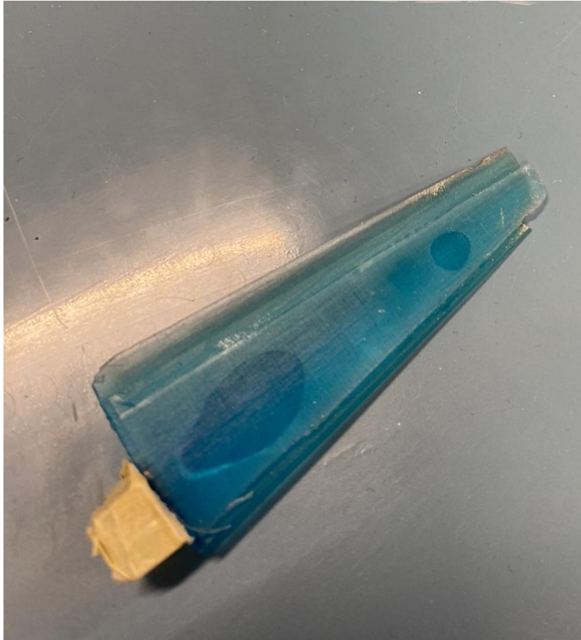
Figure 6. Broken blade resulting from high wind speeds and ineffective interfacing between the blade and the hub
