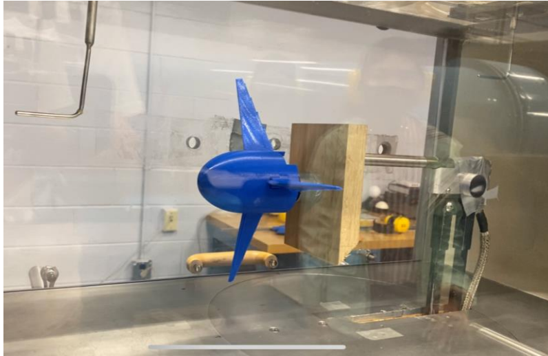
Figure 1. Version 1 of turbine in wind tunnel with larger hub and and clear deposition lines on blades
