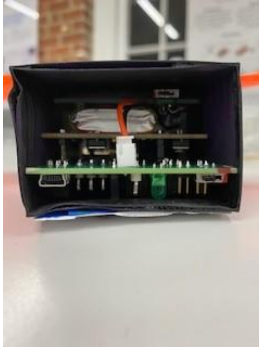
Figure 38: Close View of 3D Printed Case Interior
