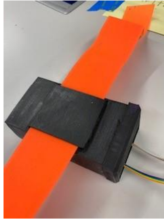
Figure 36: 3D Printed Case with Strap
