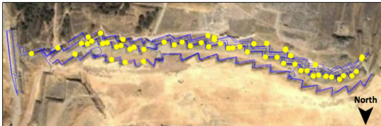
Figure 6.4: Locations of all known drainage ports (yellow circles) on the Great Walls (blue lines) (Lohr, 2014)
