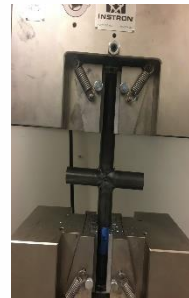
Figure 22: Tensile test setup
