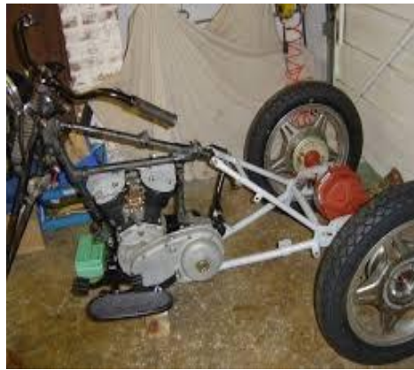
Figure 5b: Tub frame [21]
