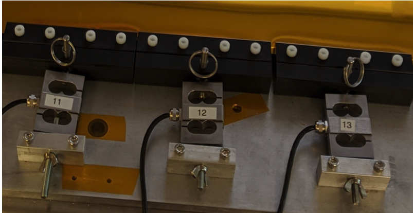
Figure 3-42: Clamps of the stretching table that are fitted with force measuring load cells.
