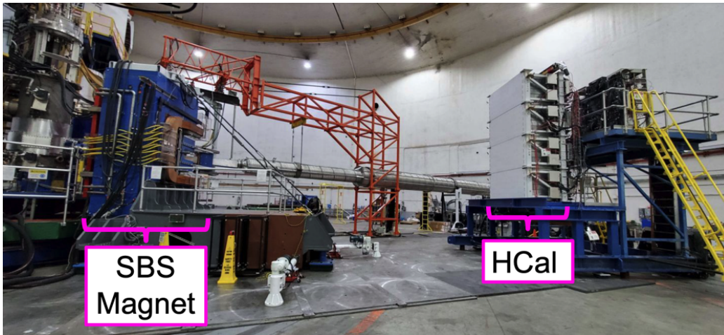
Figure 2-8: The Super BigBite Spectrometer. The SBS Spectrometer is along the scattered hadron arm and contains the Super BigBite Magnet and the Hadron Calorimeter.
