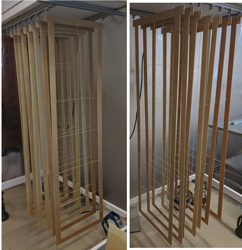
Figure 3-39: GEM frames hanging to dry in the clean room. The frames have all of their edges and corners thoroughly touched up with sand paper in order to remove any burrs, points, or sharp edges.
