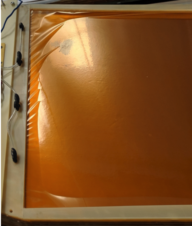
Figure 3-32: GEM chamber with non-aluminized polyimide window that has collapsed.
